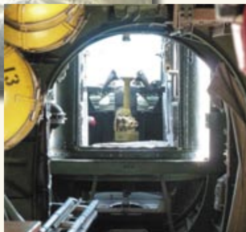
A gleaming aluminum tail turret on a restored B-24J. The gap between the turret and the fuselage let in both light and the frigid wind.
