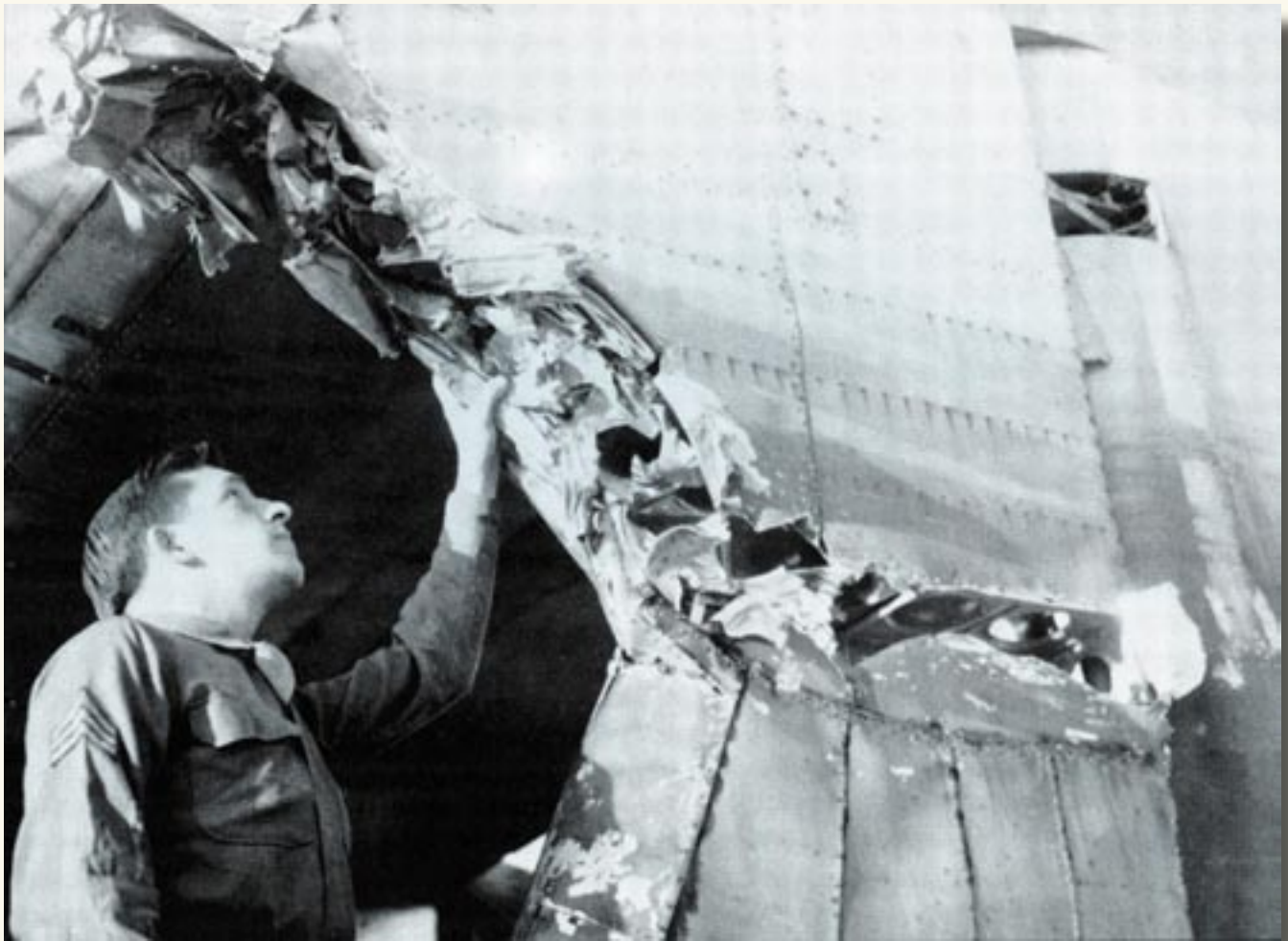
This Sargent is examining the damage done to the left rear stabilizer of Capt. Leslie's ship by the free-falling tail section of Ray's plane.
