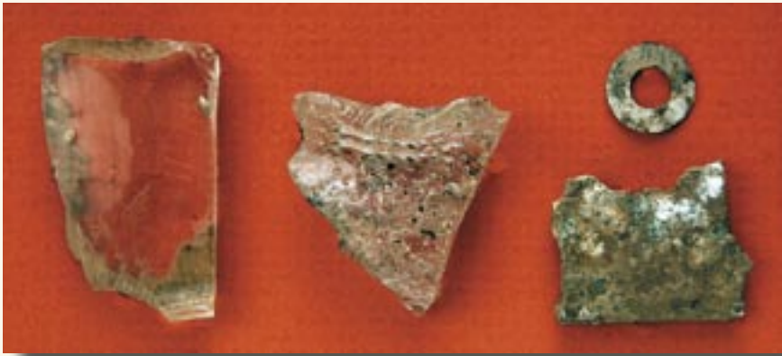
Parts of the plane, found at the crash site, including bits of aluminum and Plexiglas, one piece of which is melted and burnt.
