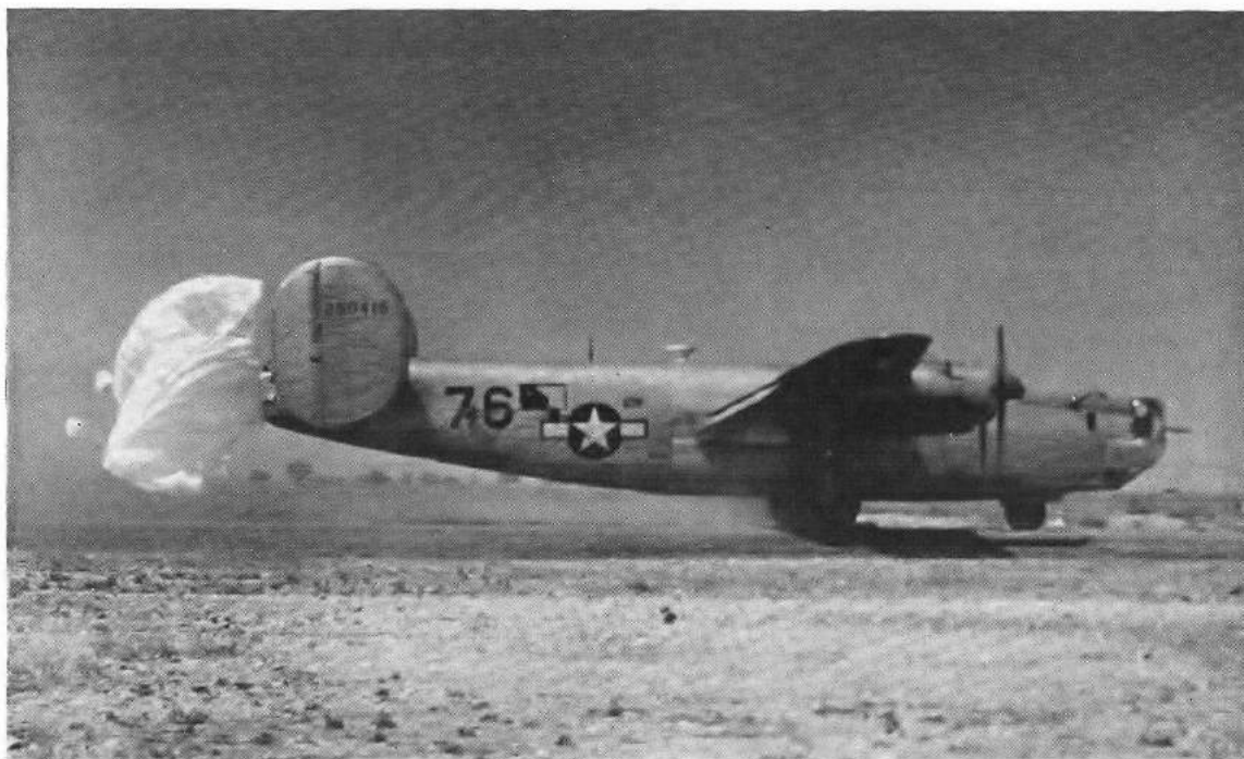
MANY OF OUR BOMBERS, crippled by enemy flak, have been forced to use this ingenious method of breaking the plane's speed on landing when brakes have been damaged. Two parachutes, tied to the waist mounts, are released as the bomber lands.
