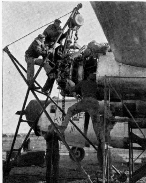
Engine-change—and 1200 new horses replace a tired engine on the wing of a heavy Liberator bomber which will be ready for the next day's flight to Munich.
